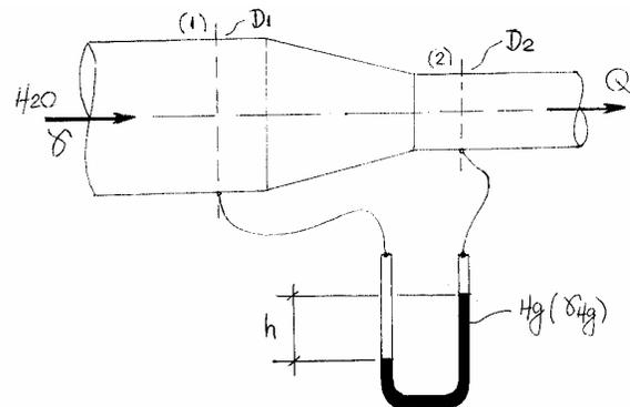
$$H_{p_{1-2}} = \frac{p_1 - p_2}{\gamma} + \frac{v_1^2 - v_2^2}{2g}$$
