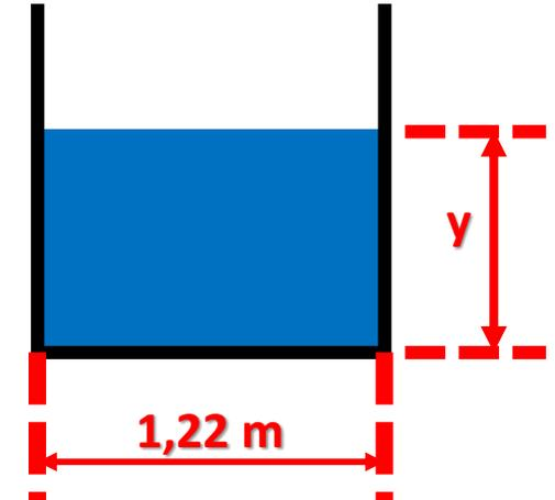
$$Q = \frac{1}{n} \times R_H^{2/3} \times I_0^{1/2} \times A$$
